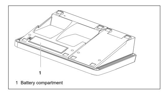
2 Place four batteries (type Mignon AA) in the battery compartment.
